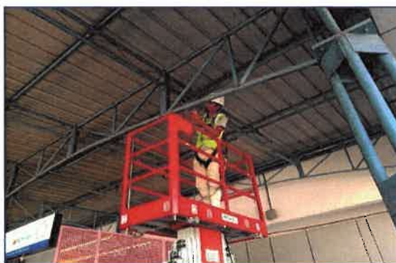
Ultrasonic Thickness Test is in Progress
