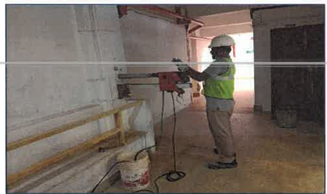
Extraction of Concrete Core Samples is in Progress
