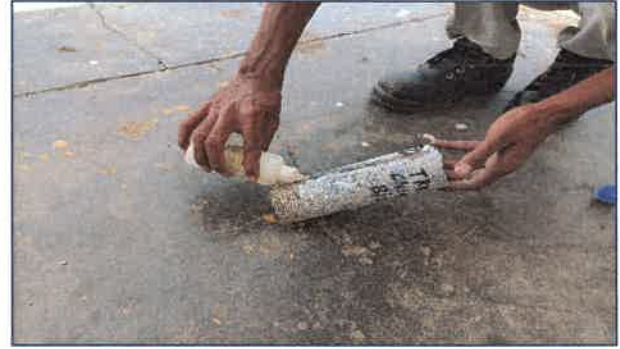
Carbonation Test is in Progress
